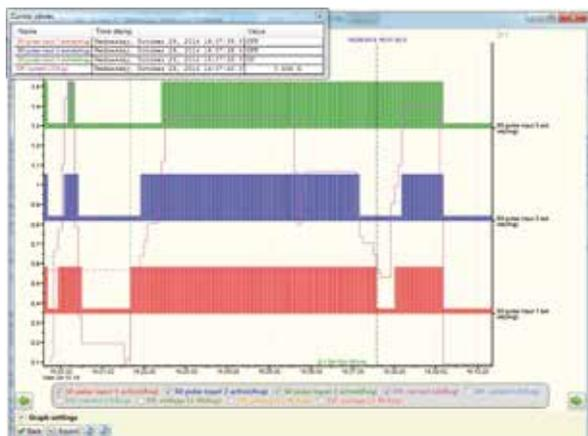
Apart from the user-defined measurements, predefined short-term measurements covering periods of 2 or 6 seconds can also be triggered, the current and voltage measurements being saved both as root-mean-square values over 10 ms intervals and as waveform curves.
