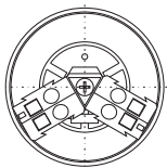
Single-phase capacitor with d = 60/70 mm Spring tension terminal AKD 25/2 for 2 \times 6 mm 2
