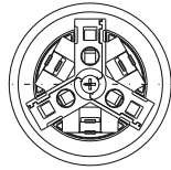
Three-phase capacitor with d = 85 mm
