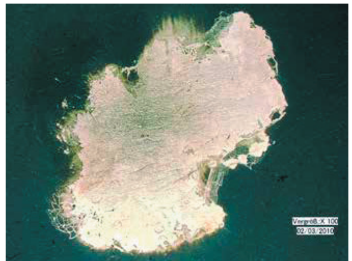
Self-healing event in typical metallized film
