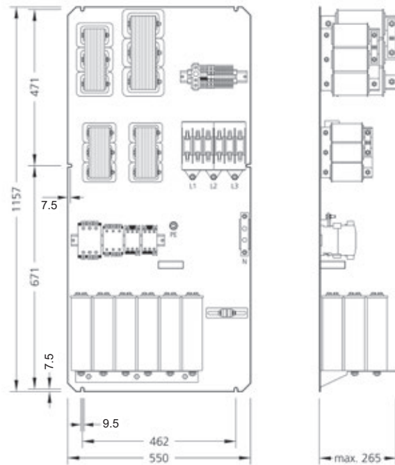
Dimensional drawing LSP-P (17.5-100 kvar)
