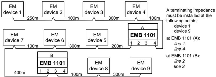
**Figure 3:** Extension of bus system
