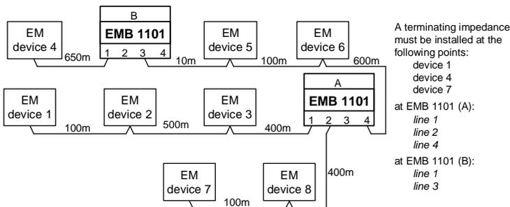
**Figure 2:** Determination of length
