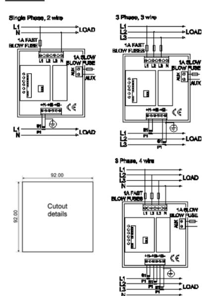
The unit may be mounted in a panel of any thickness up to a maximum of 6 mm (0.25 in). Leave enough space behind the instrument to allow for bends in the connection cables. As the front of panel enclosure conforms to IP52, it is protected from dripping water. The unit is intended for use in a reasonably stable ambient temperature within the range -10 to +55°C. Do not mount the unit where there is excessive vibration or in excessive direct sunlight.
