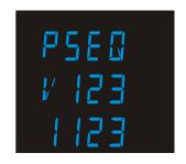
If the display shows an identical V and I sequence (123 or 132), check that the meter gives the correct forward and reverse indications. An incorrect forward/reverse indication means that all current transformer connections are reversed.
