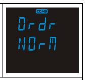
Press [V/Hz] to exit the Communications set-up screens and return to the main Set-up menu.
