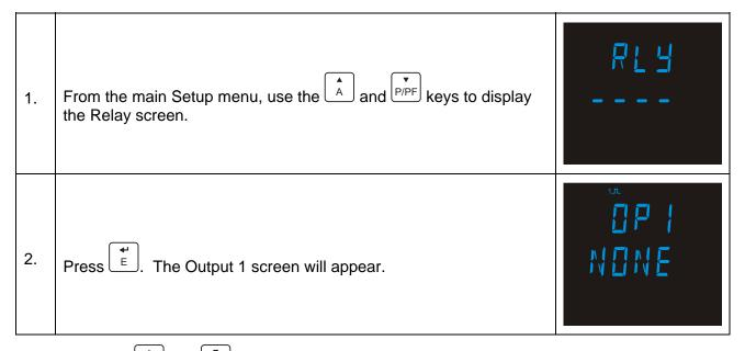
From here, the A and P/PF keys can be used to select menus for Output 1, Output 2, Rate and Pulse Width.
