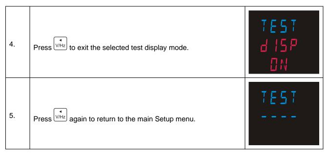
The voltage and current inputs must be greater than 5% of nominal for the test to operate reliably.
