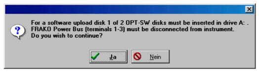
**Important!** Disconnect the instrument from the FRAKO Starkstrombus® by pulling the left connection (contact 1-3) in the contact compartment. If this is not disconnected the update will be interrupted after the transfer of the boot loader. If this should have happened follow the following instructions:
