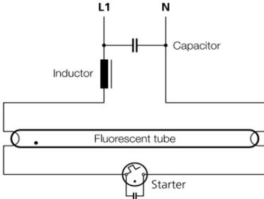
**Fig. 12:** Individual correction with the capacitor in parallel with the lamp (shunt capacitor with 230 V rating)
