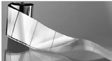
*Fig. 26: Segmented metallization*
