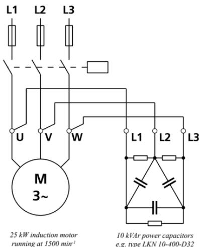
**Fig. 17:** Typical permanently installed power factor correction for a motor
