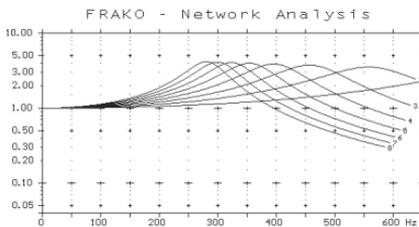
**Fig. 42:** Amplification of harmonic voltages as a function of the number of capacitor stages switched in
