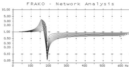
**Detuning reduces the resonant frequency to a value below 250 Hz. All harmonics above the resonant frequency of the detuned system are attenuated.**
