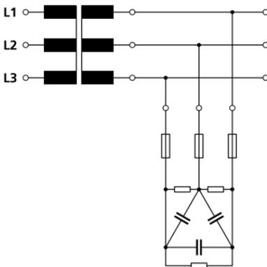
**Fig. 16:** Typical transformer with permanent power factor correction
