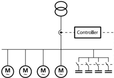
Fig. 10: Typical central power factor correction system
