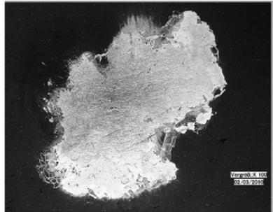
*Fig. 23: Self-healing polypropylene film*
