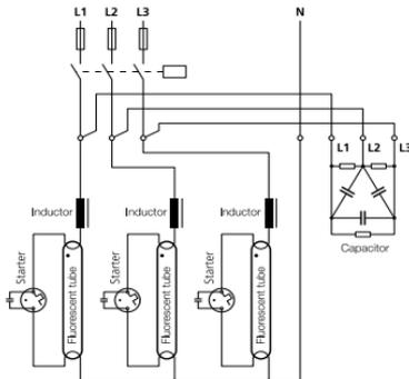
**Fig. 15:** Group correction for discharge lamps distributed between the three phases (e.g. with type LKT power capacitor)
