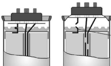
*Fig. 25: Mechanical fuse action under excess pressure*
