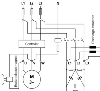
**Fig. 18:** Elevator motor with its own capacitor switching contactor and rapid discharge device
