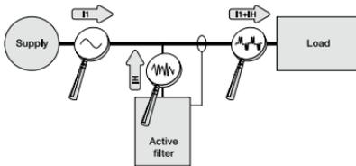
**Fig. 49:** Operating principle of the active filter
