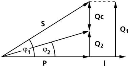
The reactive power  $Q_c$  corrected by the capacitor is given by the difference between the inductive reactive power  $Q_1$  before correction and the reactive power  $Q_2$  after correction, i.e.  $Q_c = Q_1 - Q_2$
