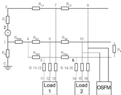
Schematic of a simulated single-phase system
