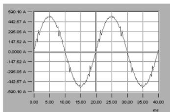
Current waveform **with** harmonic filter
