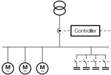
**Fig. 32: Correctly** installed current transformer registers load current and capacitor current.
