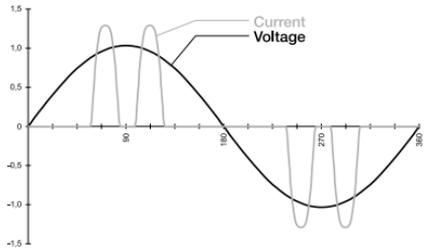
**Fig. 39:** Current and voltage in a B6 converter
