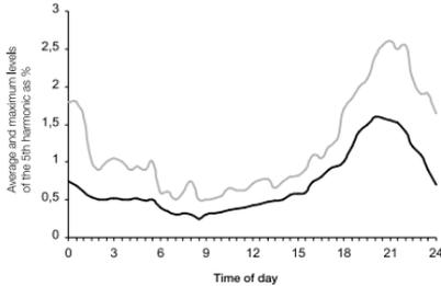
**Fig. 40:** Average and maximum levels of the 5th harmonic as % in a municipal medium voltage network
