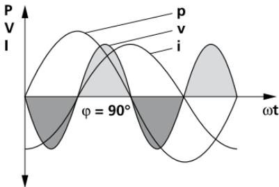
**Fig. 3:** Voltage, current and power for a purely reactive load ( $\varphi = 90^\circ$ )
