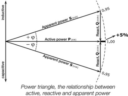
To make it at all possible for larger PV systems to feed into existing medium voltage networks, some present-day operators are even specifying power factors that can go as low as 0.90. In this case, the amount of reactive power required is equivalent to 48% of the active power. Supplying this reactive power from the PFC system can thus increase the billable active power exported by 11%!
