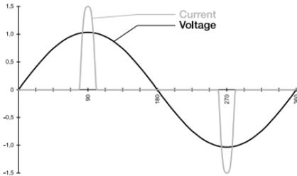
**Fig. 38:** Current and voltage in an SMPS unit
