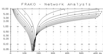
**Fig. 46:** Impedance factor  $\alpha^*$  as a function of the number of switched-in capacitor stages, with 8% detuning
