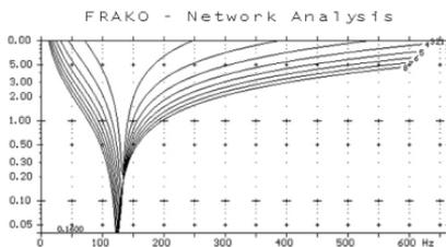
**Fig. 45:** Impedance factor  $\alpha^*$  as a function of the number of switched-in capacitor stages, with 14% detuning
