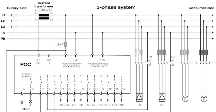
**Fig. 22:** Typical circuit diagram for a power factor correction system
