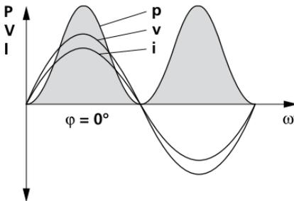
**Fig. 1:** Voltage, current and power for a purely resistive load ( $\varphi = 0^\circ$ )
