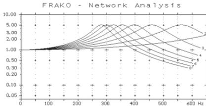
**Fig. 41:** Amplification factor for harmonic voltages in a PFC system without detuning in a low voltage network
