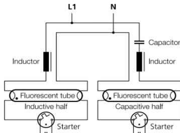
**Fig. 14:** Dual (lead-lag) circuit with the capacitor in series with one lamp, (series capacitor with 450 V rating)
