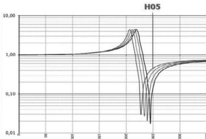
**Fig. 48:** Impedance curve for four controlled degrees of detuning
