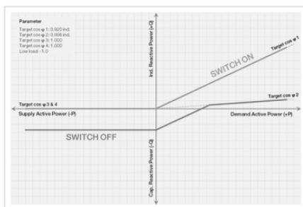
Fig. 29: Typical control characteristic curve for reduced-wear power factor correction with target cos  $\phi$  inductive when importing power but capacitive when exporting power.
