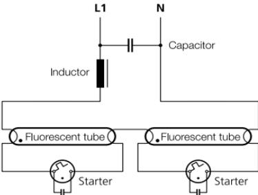
**Fig. 13:** Two lamps connected in tandem with the capacitor in parallel with them (shunt capacitor with 230 V rating)
