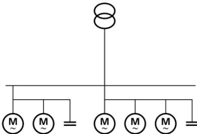
Fig. 9: Typical group power factor correction
