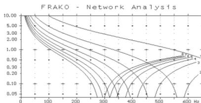
When the PFC system is fully switched in, an impedance factor  $\alpha^* \geq 0.5$  can only still be achieved for a remote control frequency of 166 Hz.
