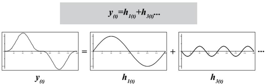
**Fig. 35:** Analysing a periodic signal into its component harmonics
