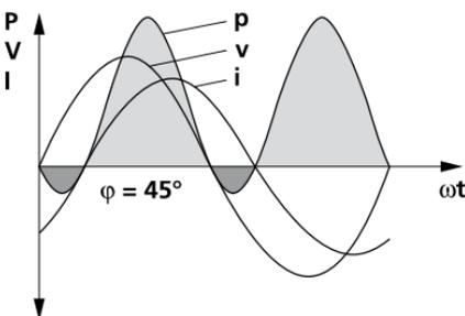
**Fig. 2:** Voltage, current and power for a resistive and an inductive load ( $\varphi = 45^\circ$ )
