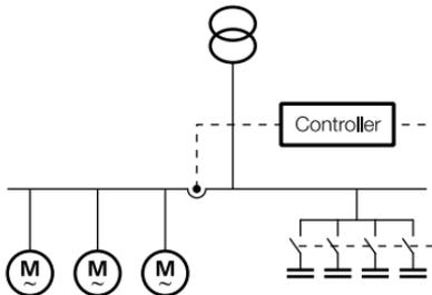
**Fig. 33: Incorrect!** The current transformer only registers the load current: the capacitor bank is switched in but not out again (no capacitor current can be measured!)
