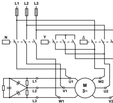
**Fig. 20:** Motor with individual power factor correction and star-delta contactor
