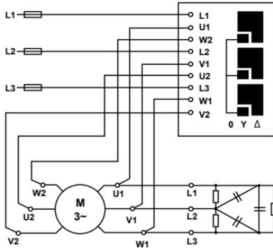
**Fig. 19:** Manually operated star-delta switch: special version for motors with individual power factor correction
