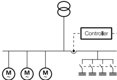
**Fig. 34: Incorrect!** The current transformer only registers the capacitor current: the capacitor bank is not switched in (no current in transformer circuit!)
