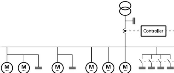
Fig. 11: Typical hybrid power factor correction system
