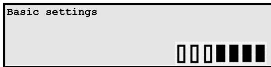
Select **Basic settings** menu item by using cursor buttons and program this by using **CR** button to enter the setting mode or the next menu level.
