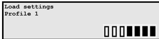
Select the profile for which the load settings are to be changed with cursor buttons and press **CR** button.
