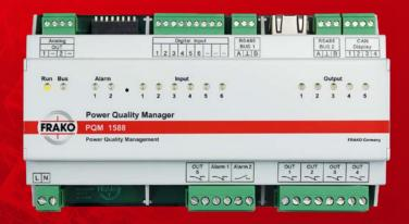
Whether to inform, to alert or to connect: the FRAKO Power Quality Manager is a multitalent, an all-in-one instrument. Using interfaces such as OPC UA and REST, it becomes the focal point of your Industry 4.0 communications and your gateway to the Internet of Things (IoT). The FRAKO PQM makes it child's play to integrate machinery and industrial plant into higher-level control systems and to transfer data to cloud-based analysis solutions.
