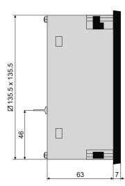
The PQA is designed for mounting in a 138 mm  $\times$  138 mm cutout to IEC 61554 in the front of a control cabinet. It is held in place by four retaining lugs in the corners of the instrument.
