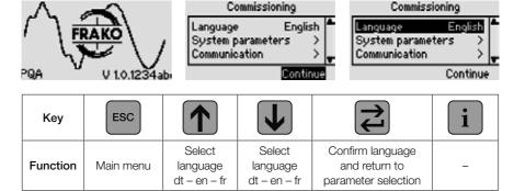
When the power is switched on, the Start screen is displayed, showing information about the installed firmware. The initial start-up dialogue then starts automatically, in which the essential parameters for operation can then be set and the start-up mode selected.
