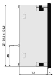
The PQC is designed for mounting in a 138 mm x 138 mm cutout to IEC 61554 in the front of a control cabinet. It is held in place by four retaining lugs in the corners of the instrument.
