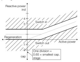
An effective combination of "parallel shift" and "limitation" is illustrated in the following diagram:
