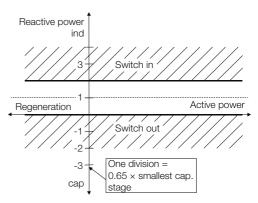
Control characteristic at  $\cos\,\phi_{target}=0.92\,\text{ind}$  Limitation=OFF  $Parallel\ shift=-1.0\ (capacitive)$
