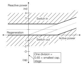
For the sake of completeness, the following diagram shows the characteristics of the control band when set for a capacitive cos  $\phi_{target}$ . In this case, the control range does not extend laterally at the reactive power axis into the regeneration quadrants, but is mirrored from the power draw side into the regeneration side.
