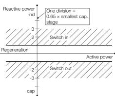
Control characteristic at  $cos \; \phi_{target} = 0.92 \, ind \\ ind \; Limitation = 0 \\ Parallel \; shift = 0$
