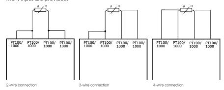
In addition, one or two 2-wire NTC probes (Article No. 29-20094, 7-metre cable) can be connected as shown below:
