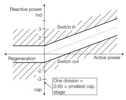
to the supply network) can be seen. The 'kink' in the band (characteristic line) is not reflected in the regeneration quadrants. Instead, the band extends laterally from the point where it crosses the reactive power axis (y axis).
